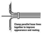
Parallel hose lines may be clamped together to improve appearance and function. Although the hose assemblies are, in a sense, operating together, each line is subject to its own impulse surges and other movements. Care must be taken so that relative movements of the assemblies will not cause the securing clamps to abrade the sleeve or hose. For example, high pressure and low pressure lines generally should not be clamped together as they tend to react differently in operation.
