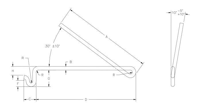
FIGURE 1. Clip, locking, turnbuckle.
