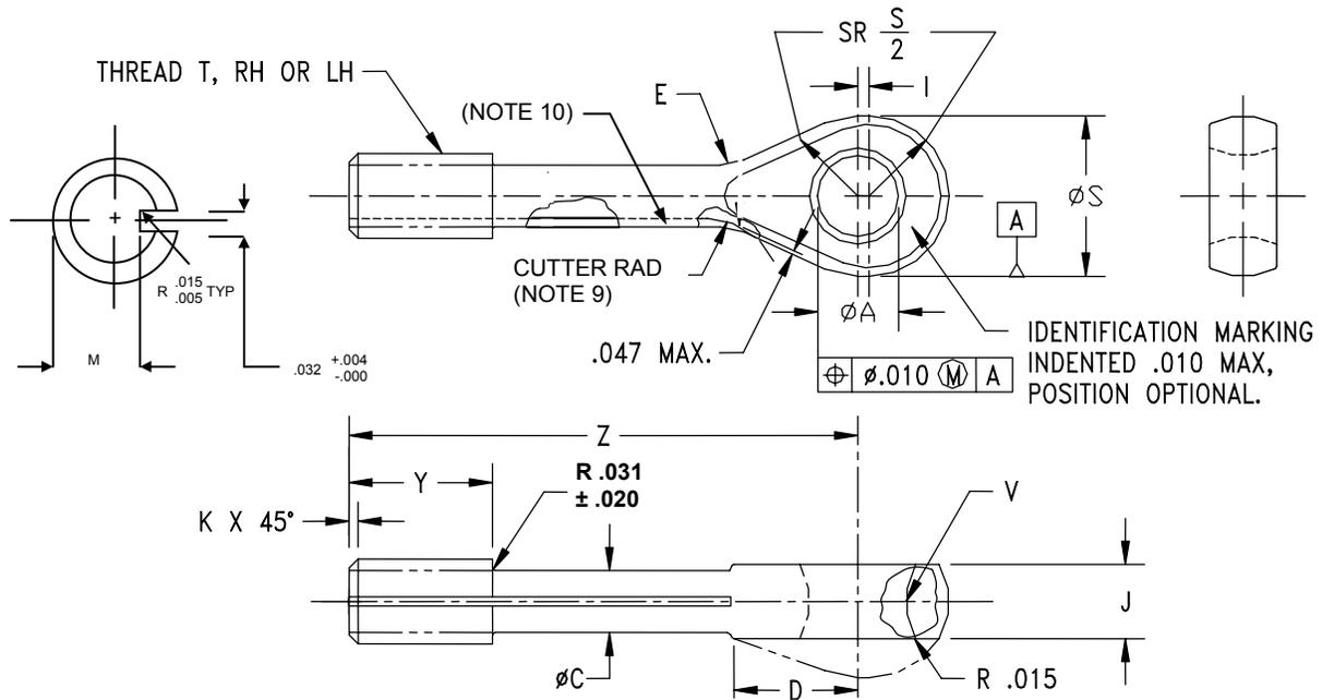
FIGURE 1. Eye end, turnbuckle, clip locking (for wire rope).
