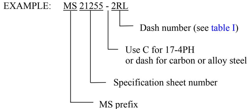
MS21255C2LS Indicates - Eye, turnbuckle, 17-4PH, 0.1380 (#6)-40, left hand thread, short.
