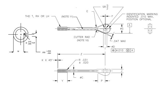
FIGURE 1. Eye end, turnbuckle, clip locking.
