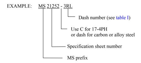
MS21252C3LS Indicates - Clevis end, 17-4PH, 0.1900 (#10)-32 left hand thread, short. MS21252-3RL Indicates - Clevis end, steel, 0.1900 (#10)-32 right hand thread, long.
