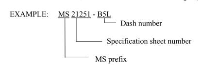
MS21251-B5L Indicates - Body (barrel), turnbuckle, brass, 0.2500 (1/4)-28 thread, long.
