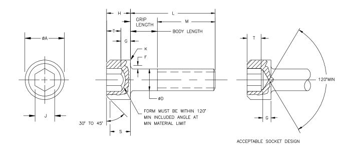
FIGURE 1. <u>Dimensions and configurations</u>.
