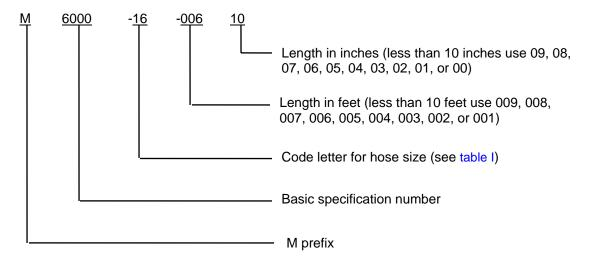
PIN example: M6000-H-00610 describes a 1-inch inside diameter hose that is 6 feet 10 inches long.
