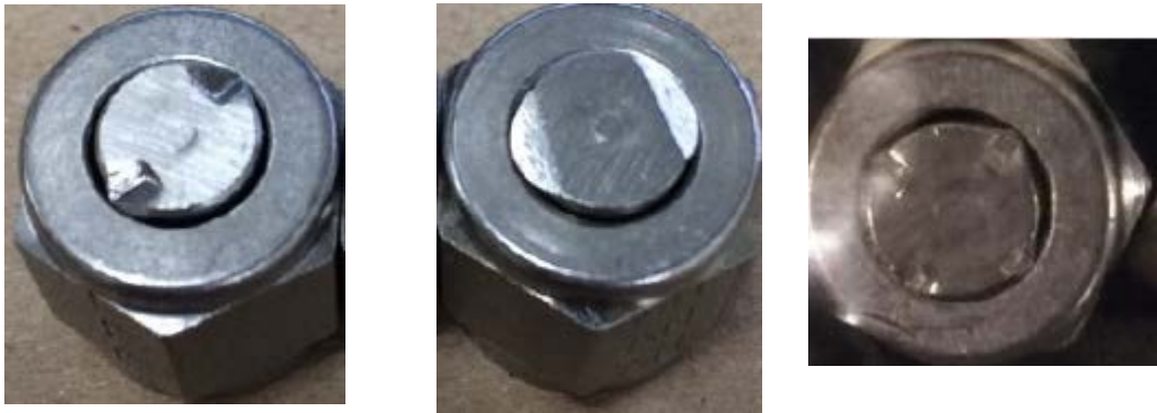
FIGURE 4. Examples of approved methods of cap retention.
