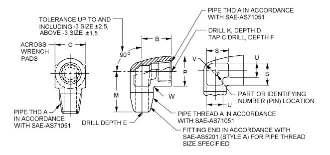
FIGURE 1. Elbow 90° dimensions and configuration.
