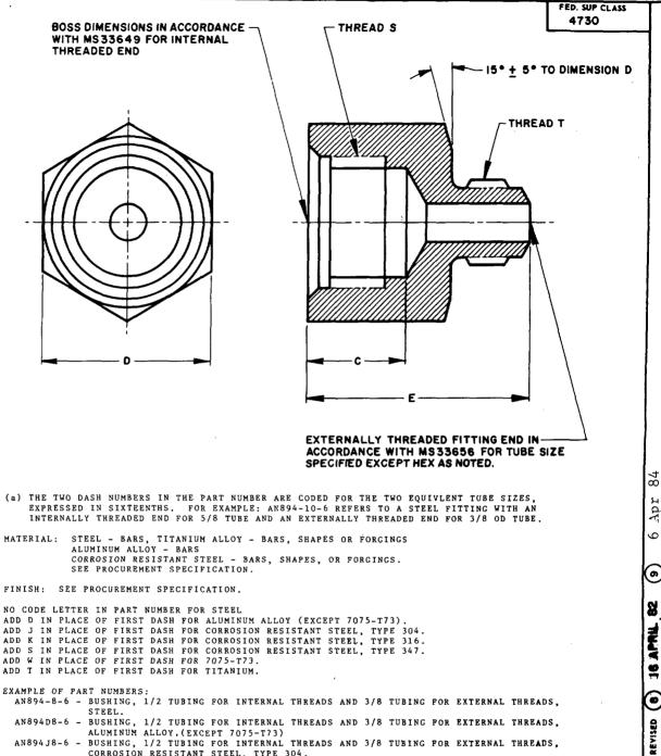
AN894D8-6 - BUSHING, 1/2 TUBING FOR INTERNAL THREADS AND 3/8 TUBING FOR EXTERNAL THREADS, ALUMINUM ALLOY. (EXCEPT 7075-T73)
